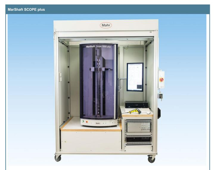
The MarShaft SCOPE plus is a universal, fully automatic, optical measuring unit for measuring turned parts.
