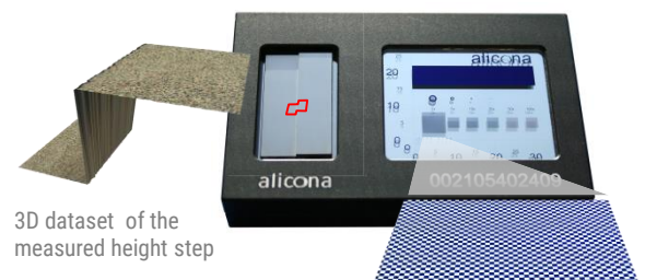
Chess pattern for the verification of lateral measurements
