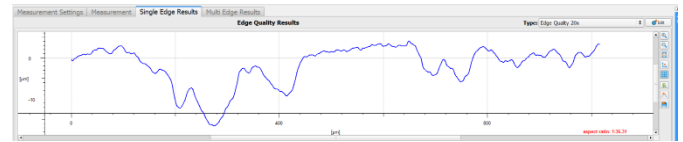
Extracted surface profile along the edge
