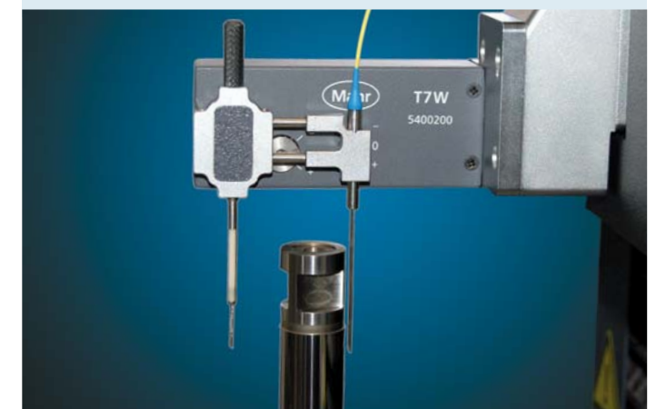
Left the tactile probe, right in the picture the optical sensor in use on the testpiece
