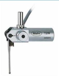
The inductive **T2W** probe is a universal device. The fact that the probe arm can be moved in a 180° range and that there are a variety of clamping possibilities for the probe, means that measurements can also be performed on difficult to access areas. You can combine easily exchangeable probe arms with a variety of styli in order to adapt the probe to the relevant measuring tasks or workpieces.
