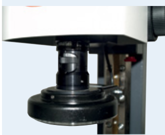
Six step Navitar Zoom lens-Objektiv with 0.7-4.5x magnification
